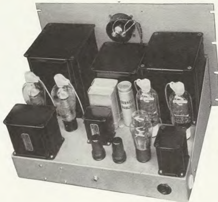
TOP VIEW SPEECH AMPLIFIER, MODULATOR AND HIGH VOLTAGE POWER SUPPLY
